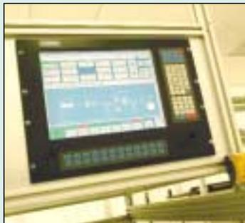
Three work stations are located at the beginning, middle and end of the line and instead of manually turning the pods, workers now have complete control from touch screens. And because they are Windows based the computers are user friendly and simple to operate. The automated controls enable line supervisors to quickly adjust and manipulate the line mechanics produced. The data base can change the controls to work with specific styles of media, the width, loft and weight of each filter.
